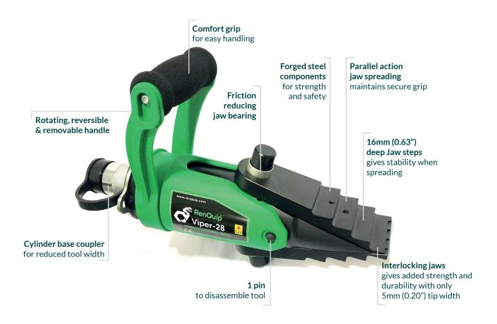
The Viper-28 is RenQuip's latest revolutionary Flange Spreading Wedge – capable of entering a 5mm access gap and producing a spreading force of 277kN (27.7T) per tool yet weighs only 5Kg (11lbs).
